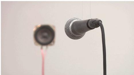
Audio feedback, also known as Larsen effect, is a special kind of positive loop gain which occurs when a sound loop exists between an audio input (for example, a microphone or guitar pickup) and an audio output (for example, a power amplified loudspeaker).
